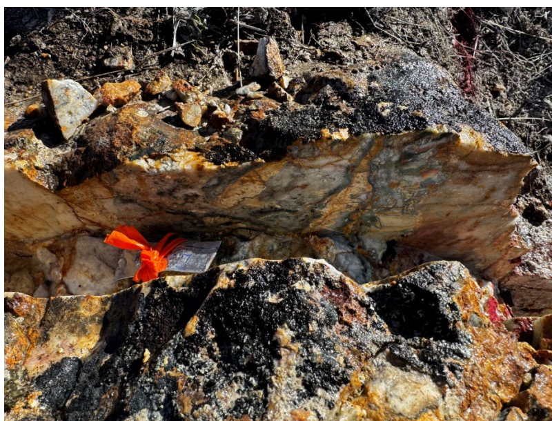
Figure 16. Sawn Channel sample showing epithermal textures within the vein. Sample ID CC278, returning 1.6m @ 333g/t AgEq (136g/t Ag & 2.4g/t Au) or 4.0g/t AuEq. Looking North. Refer ASX release dated 2 December 2025.
