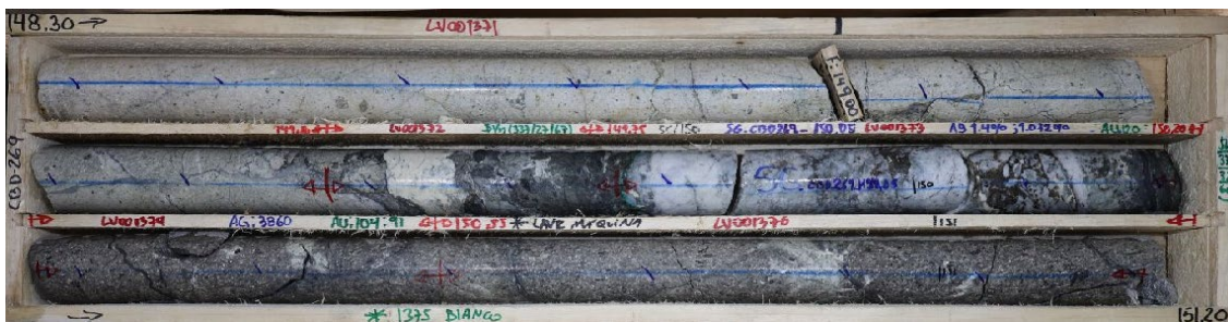
Figure 7. CBD269 Temer Main mineralised shoot quartz breccia, 0.8m @ 4,131g/t AgEq from 149.75m to 151m. Refer to Andean ASX release dated 11 December 2025.
