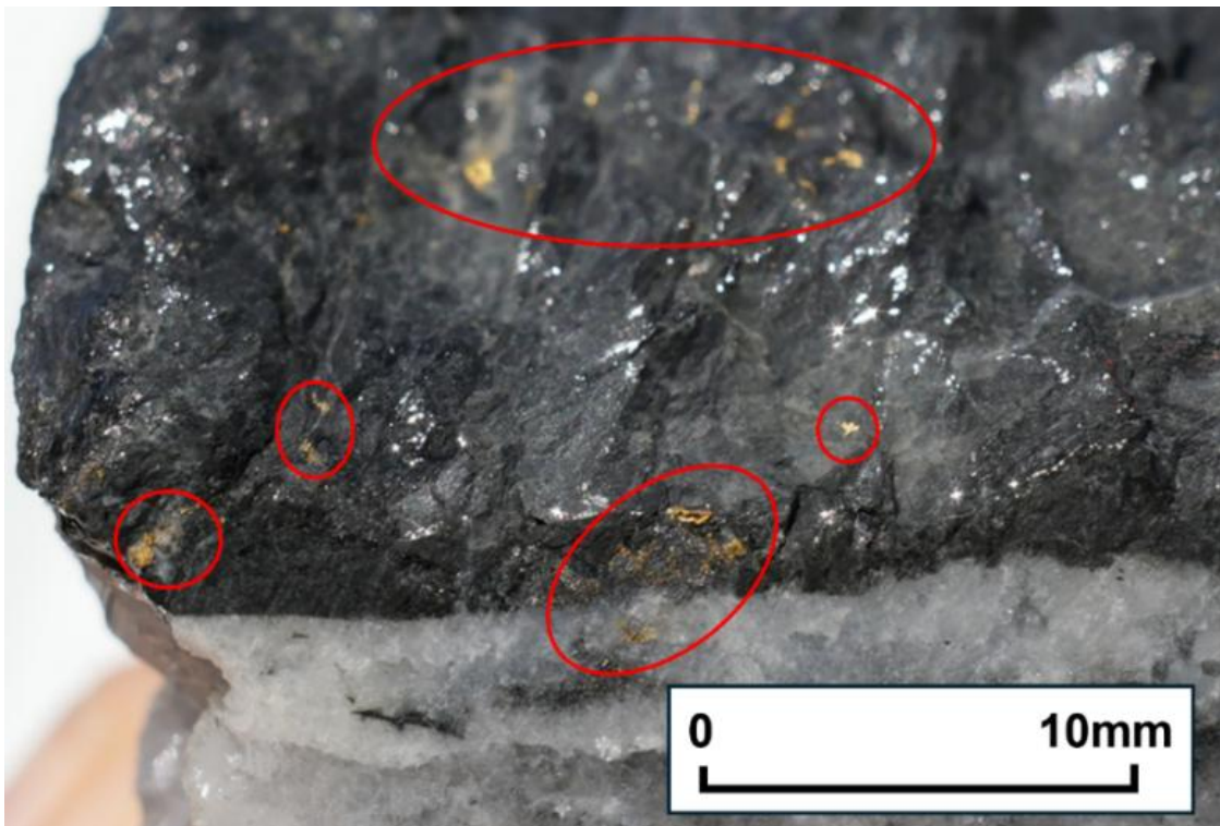
Figure 7 BMDD004W1 showing visible gold (red circle) in a quartz carbonate vein at 635.4m (downhole depth)
