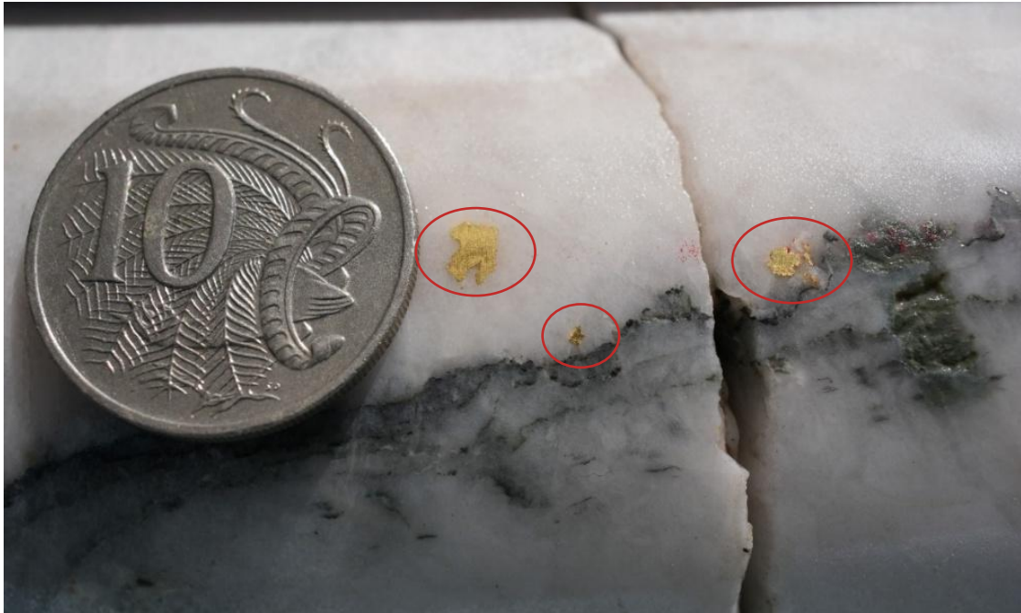
Figure 6 BMDD003 showing three occurrences of visible gold (red circles) in a stylolitic quartz carbonate vein at 607.6m
