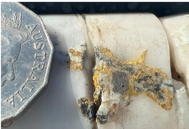
Figure 4 BMDD001W1 – visible gold at 544.6m in intercept 1.2m @ 543g/t Au from 544.2m
