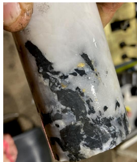
Figure 5 BMDD001W1 – visible gold at 544.9m in intercept 1.2m @ 543g/t Au from 544.2m
