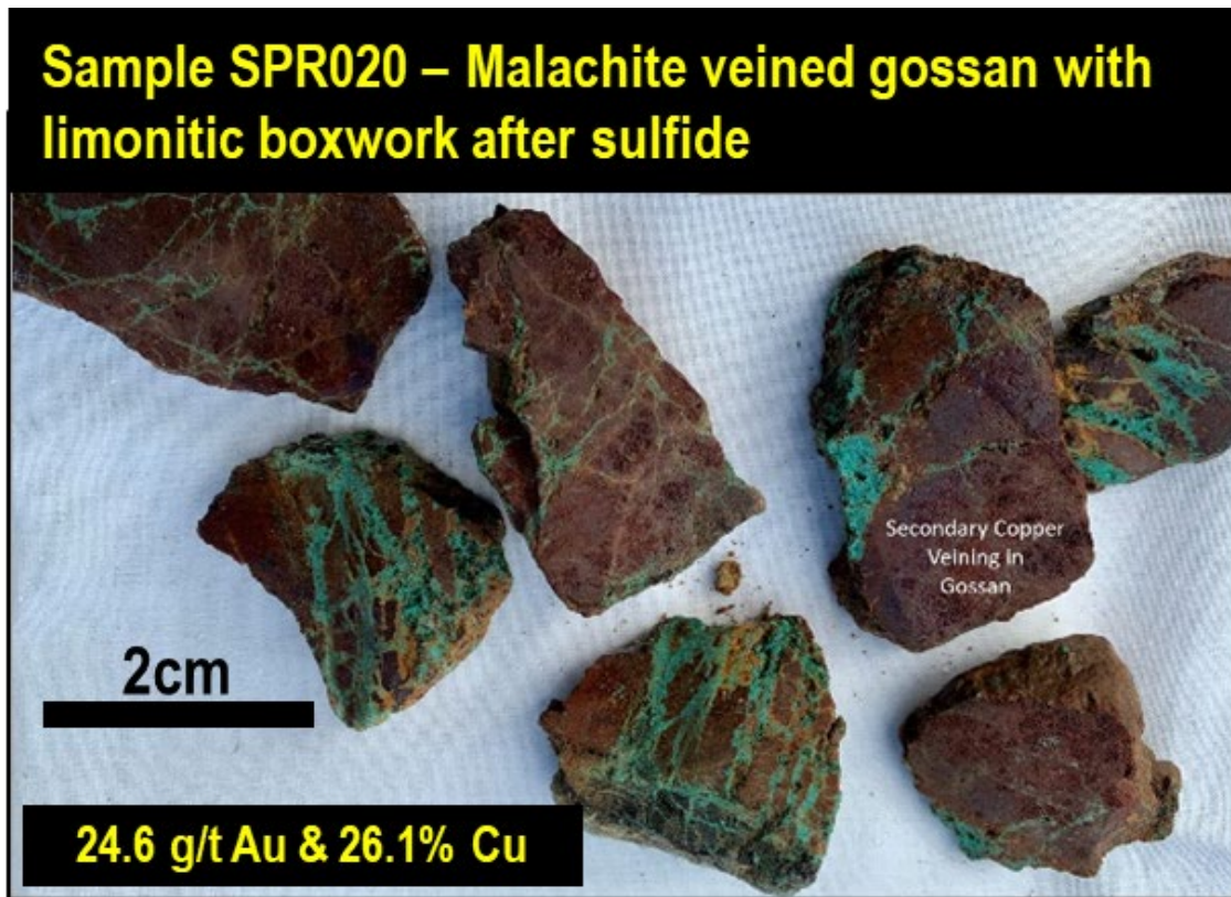
Figure 5: Mullock sample of malachite veined gossan with limonitic boxwork after sulfide (Sample SPR020) (ASX: SLZ 20 May 2020).
