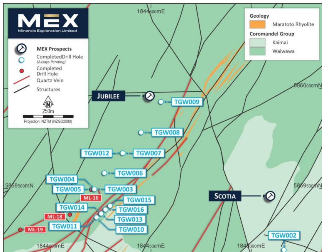
Figure 4: Jubilee drilling program is designed to target historical high-grade zones
