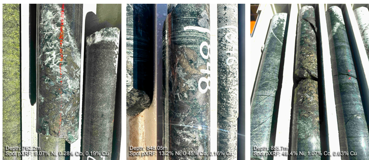
Figure 5: Photos showing examples of semi-massive sulphide segregations and globules in hole MTRC011 Note: core is NQ2 being 2 inches or 50mm diameter
