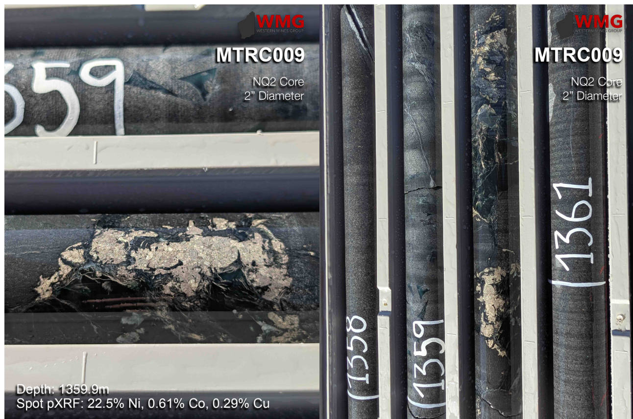
Figure 7: Photos showing examples of sulphide segregations in hole MTRC009 (EIS9) Note: core is NQ2 being 2 inches or 50mm diameter
