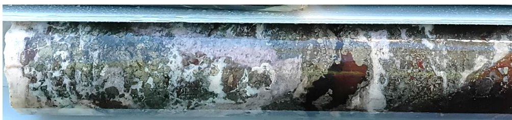
Figure 1. Sulphide-hematite-quartz-carbonate breccia that forms part of the broad mineralised interval in YQ-26-018. This interval graded 0.74m at 572g/t Ag & 10.0g/t Au from 354.64m.
