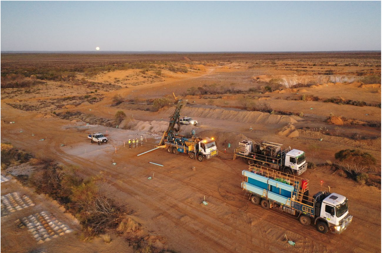
Figure 5: Stage 2 Grade Control RC Drilling at Iguana
