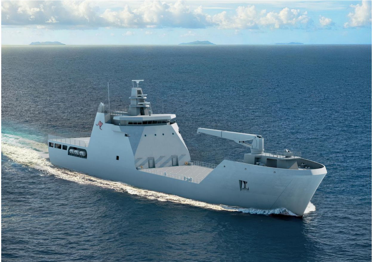
Eight, 100 metre Landing Craft Heavy vessels will be constructed by Austal in Henderson, Western Australia, based on the Damen LCT100 design (image: Austal)
