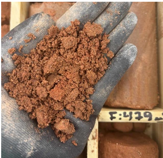
Figure 1. Core extracted at 479m show highly porous sandy sediment soaked in brine – RHS drill team
