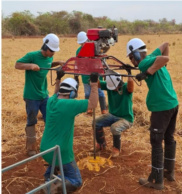
Figure 2. Auger drilling at Santa Anna Project 19 January 2026.
