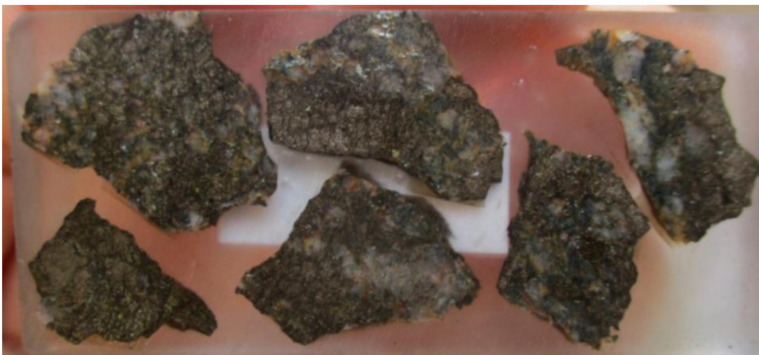
Figure 5: Sample 41 of appendix B ASX: PMM 01/12/2025 shows the clastic material in this sample is composed of transparent medium-grained quartz, small, black-coloured flakes interpreted as biotite, and light orange to pink-coloured blocky scheelite grains. These clasts sit within a matrix composed entirely of pyrrhotite.
