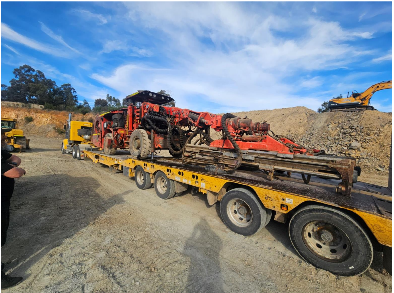
Figure 3. Twin Boom Jumbo delivered to Union Hill
