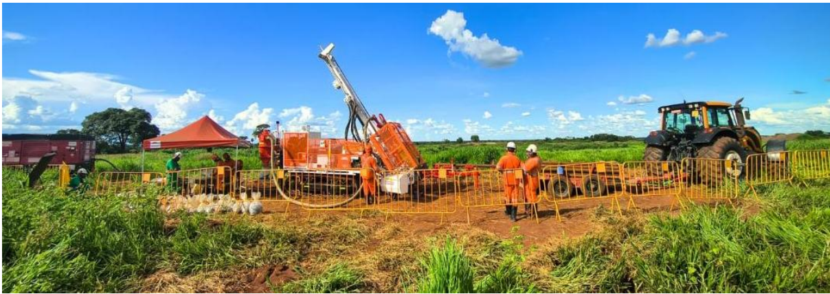
Figure 1: RC drill rig operating at the Santa Anna Project, Brazil
