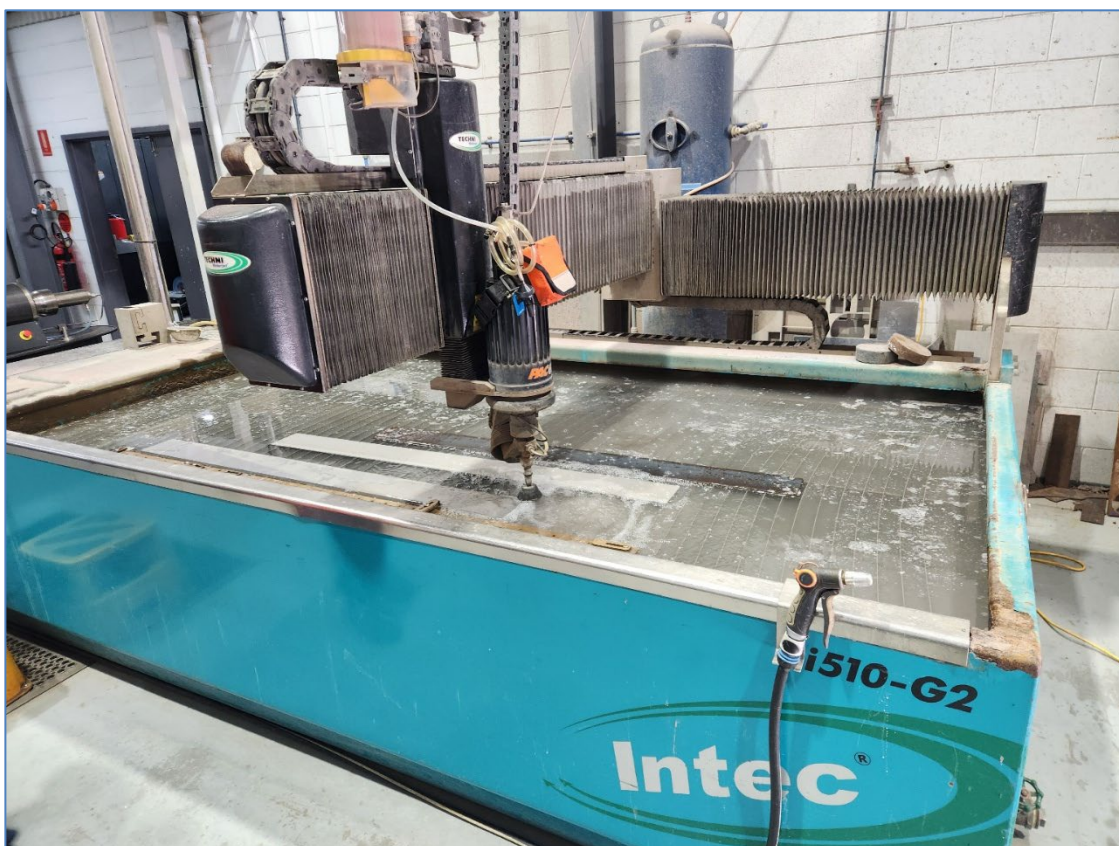
Figure 9 – CSIRO Queensland (Engineering Workshop) Technijet - Intec 510-G2 waterjet cutting machine
