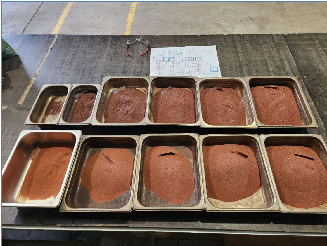
Figure 8 – IHC samples of Industrial Waterjet Cutting Garnet, derived from the Kanmantoo Mine live tailings stream.
