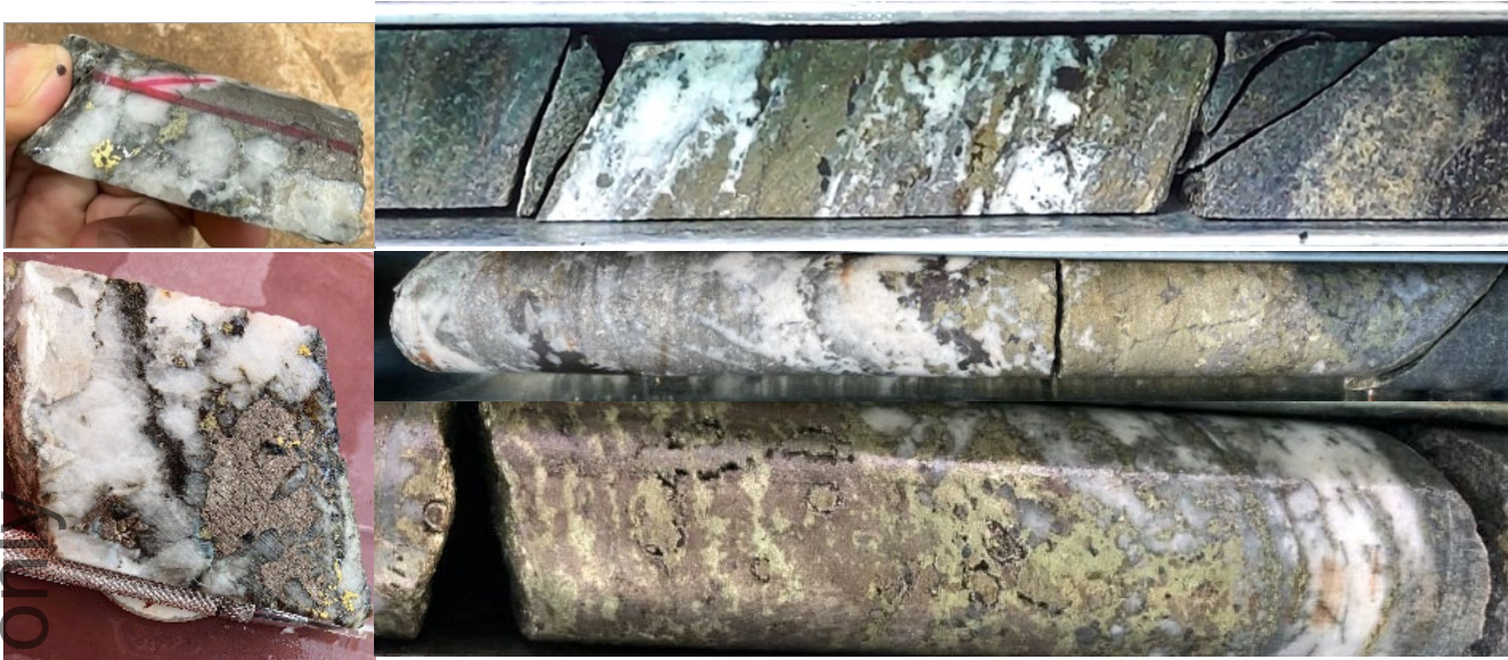
Figure 6 | Mineralised veins in Memot diamond core. Quartz veining with Pyrite, Arsenopyrite, Pyrrhotite, Chalcopyrite and Sphalerite sulphides. Left Hand Side photos: DD24MMT243 - 1m @ 2,090.00g/t Au from 130m. Right Hand Side top to bottom DD21MMT001 - 1m @ 8.91g/t Au, 2.16% Cu from 48m, DD22MMT013 - 0.4m @ 17.70g/t Au, 230g/t Ag, 2.78% Cu, 0.56% Pb and 1.74% Zn from 190m and DD21MMT006 - 1m @ 25.4g/t Au, 73g/t Ag, 1.81% Cu, 0.1% Zn
