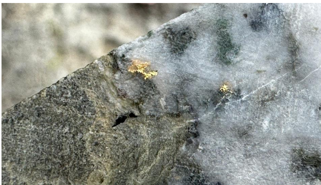
Figure 1. Coarse visible gold (yellow) up to 4mm across associated with a newly discovered quartz vein structure intersected in AMD016 immediately to the east of Happy Valley. This interval graded 0.6 metres at 66.7g/t Au from 51.3m.
