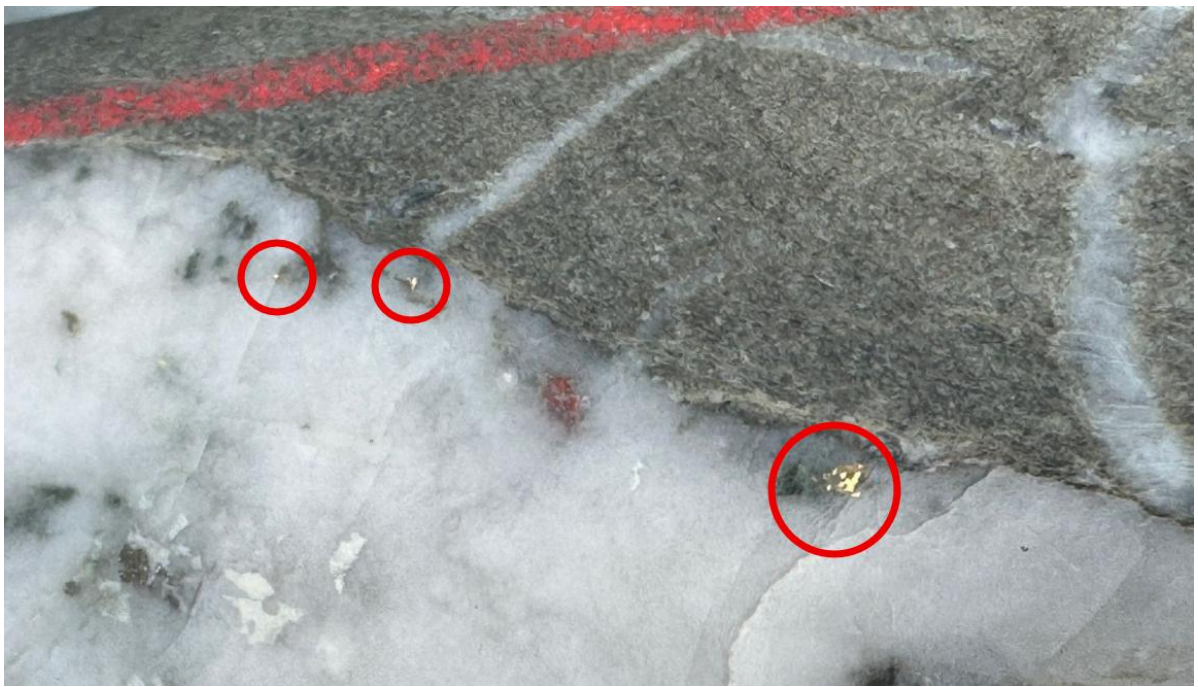
Figure 3. Further visible gold (highlighted) up to 2mm across associated with a newly discovered quartz vein structure intersected in AMD016 immediately to the east of Happy Valley. This interval graded 0.6 metres at 66.7g/t Au from 51.3m.
