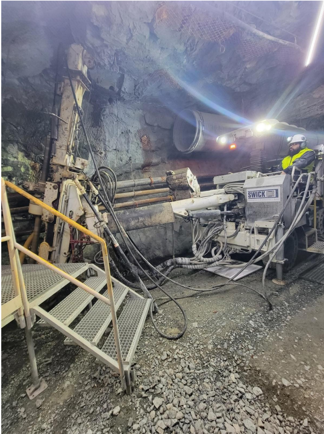
Figure 1: Diamond Drilling at XC4- drill hole DDH256.
