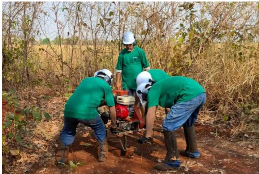
Figure 2. Auger drilling at Santa Anna Project
