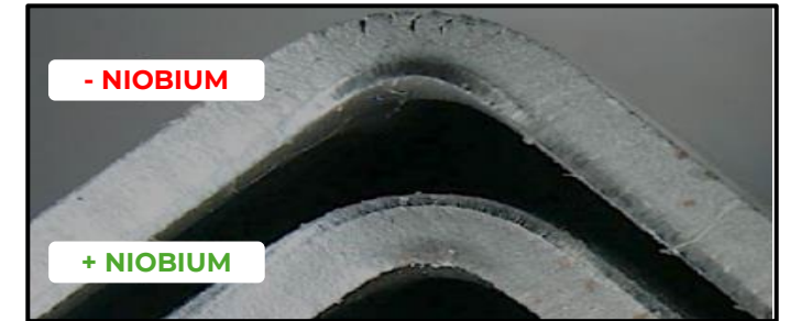
IMPROVED FLAT SHEET FORMABILITY WITH NIOBIUM 4
