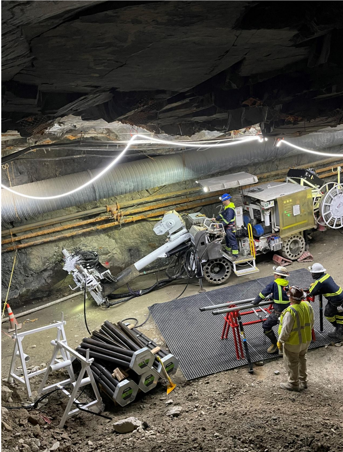
Figure 1: Swick Gen II underground diamond drill rig, drilling DDH251 at crosscut 3 (XC3).
