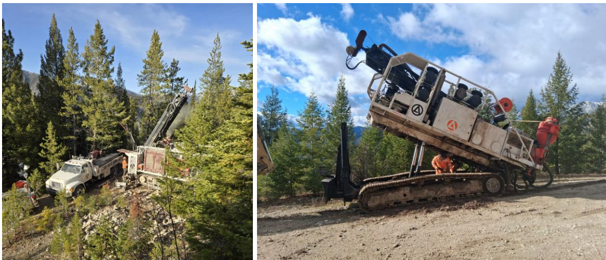
Figure 2: LEFT: Photo of the RC drill rig on site at Golden Gate. RIGHT: A photo of the RC rig that will drill the three holes at Golden Gate, a track-mounted RC1500.
