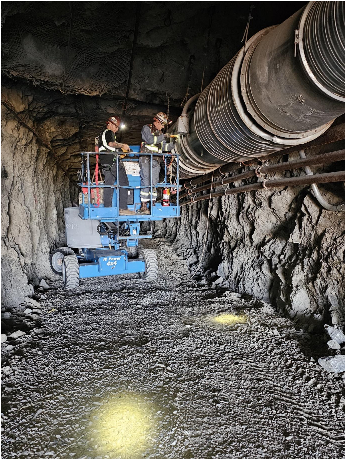
Figure 5: Recently purchased 4x4 articulated boom performing checks on ventilation fan at Stringbean Alley Decline portal. The work platform provides a stable platform as the Company advances pumping equipment and drops ventilation at the water interface.
