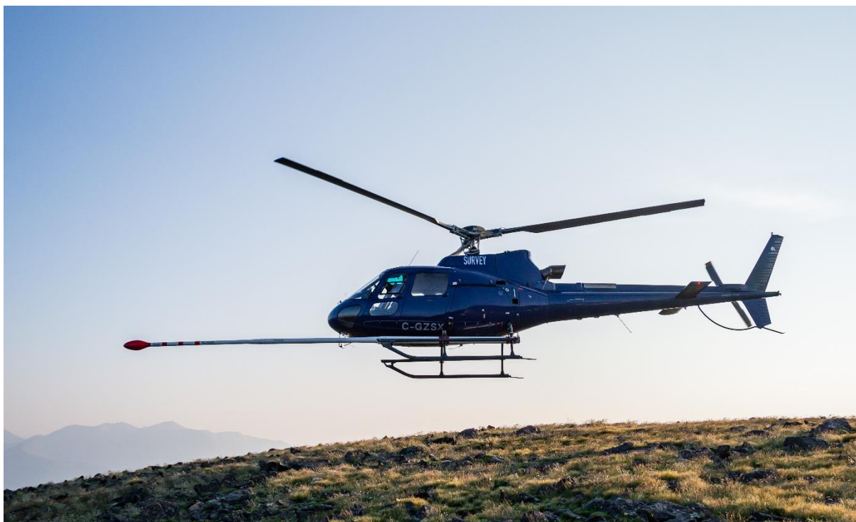
Figure 1; Photo of Eurocopter AS-350 B3 with magnetometer probe being utilised at Locksley's Mojave Project.
