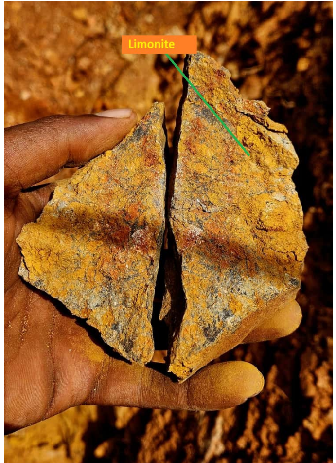
Figure 7: Strong limonitic alteration from oxidised copper sulphides from sample L4480
