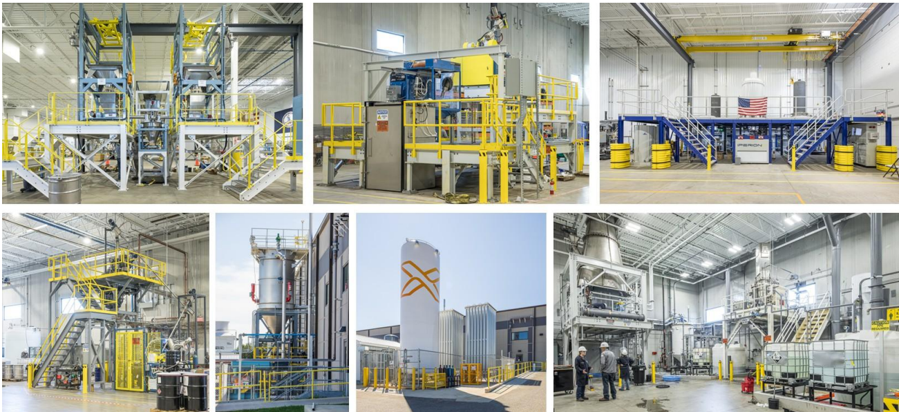
Figure 2: Various operations, including clockwise from top left – reagent mixing, crucible loading / unloading, HAMR furnace operations, product leaching, argon facilities, product collector, jet mill operations
