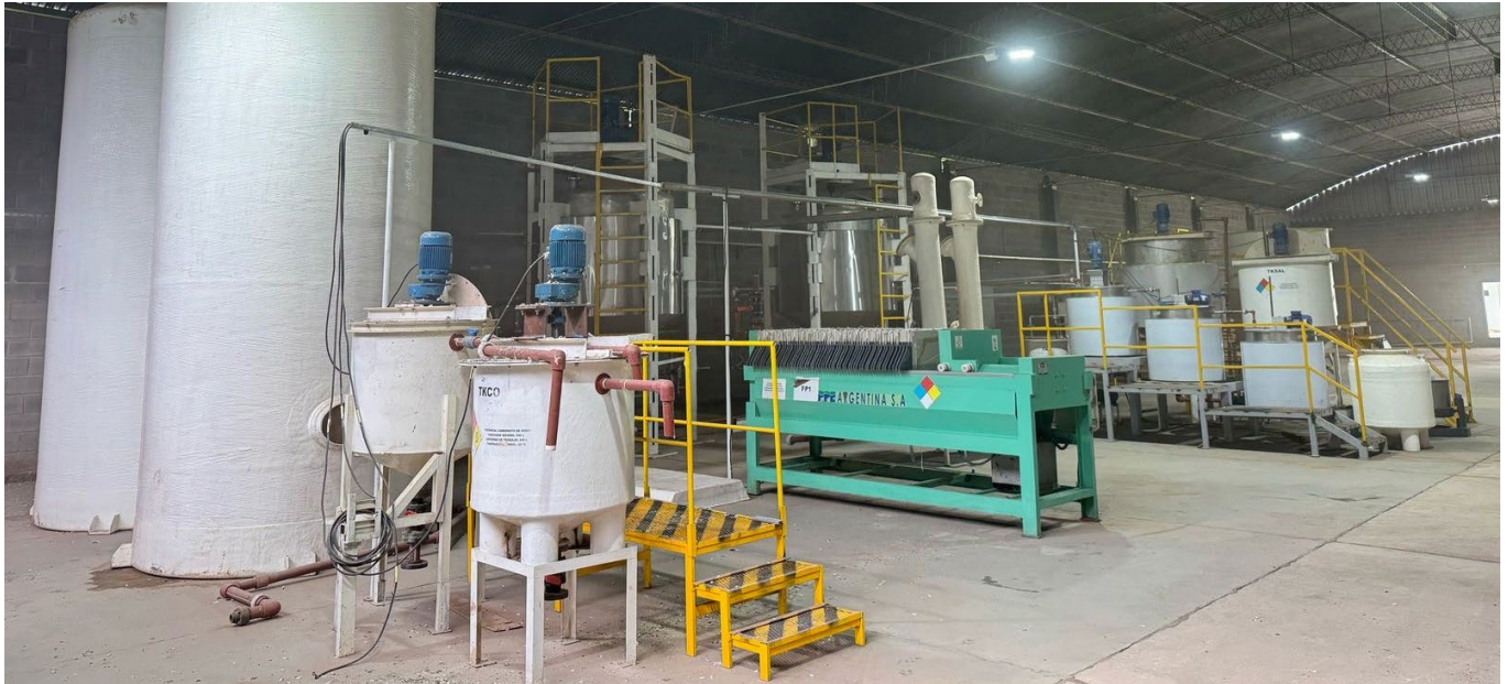
Figure 3: Pursuit's 250tpa Pilot Plant producing Lithium Carbonate in Salta, Argentina.
