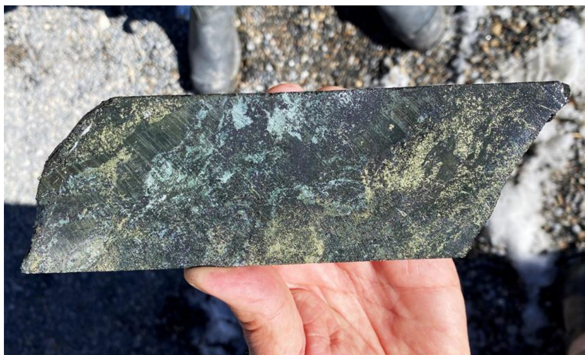
Figure 1: Cu-Au-Ag-In-Ga rich mineralisation in drill core from approximately 422m (1,385ft) downhole in WD22-01c (see Table 8 for interval details).
