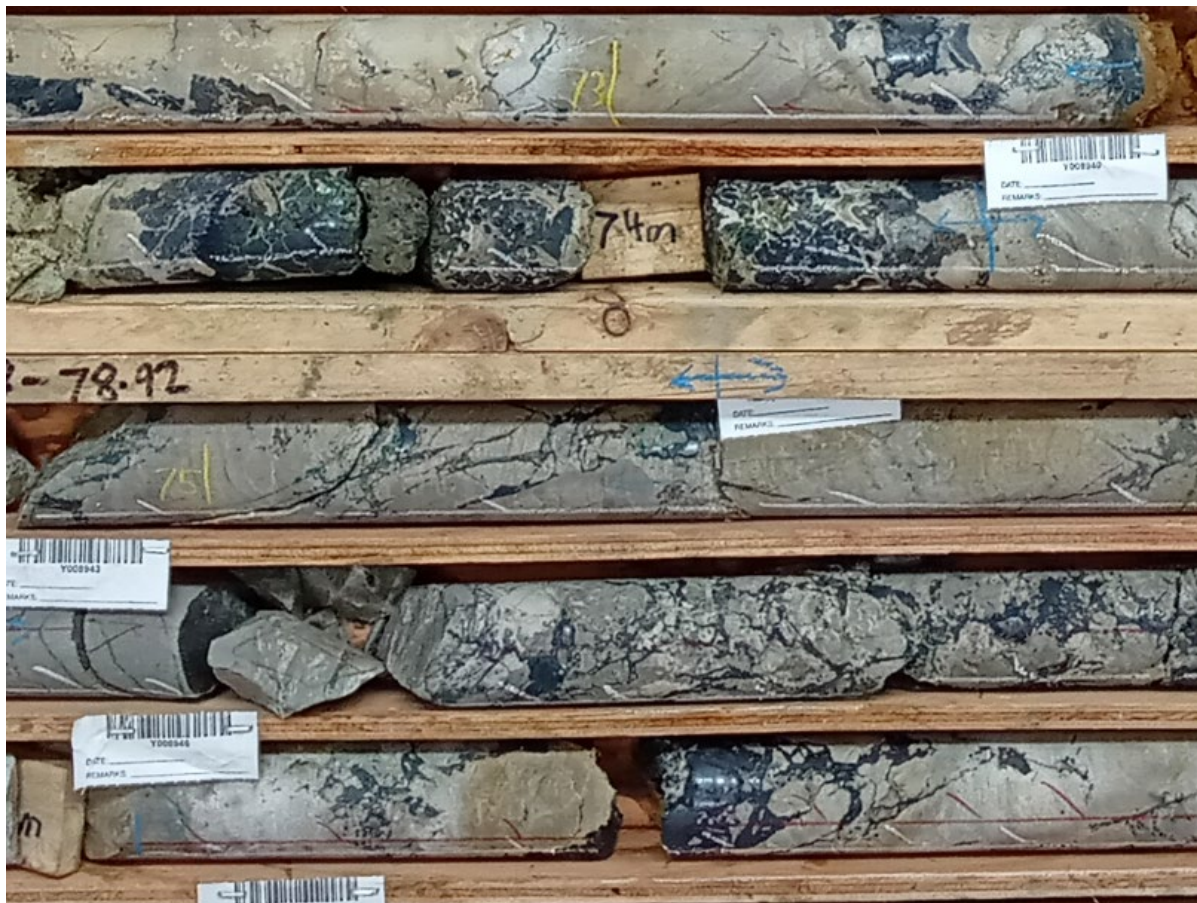
Figure 4: Dense semi-massive and breccia visual chalcocite (dark grey mineral) from PFS-002 (72.7–76.5m downhole). This interval assayed at an average grade of 8.1% Cu, 31g/t Ag.
