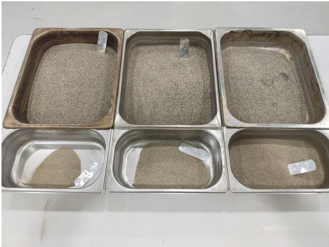
Plate 2 – Construction sand from large scale pilot plant operation tested for asphalt and concrete applications
