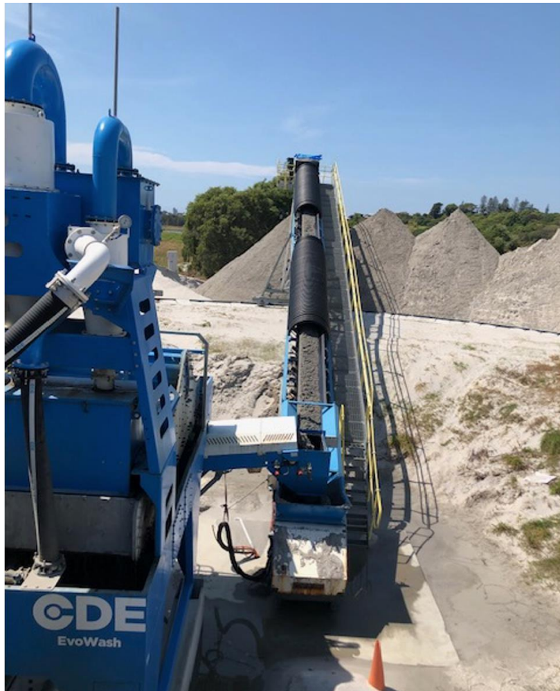
Plate 5 - Dewatered sand stockpiles and mobile stacker
