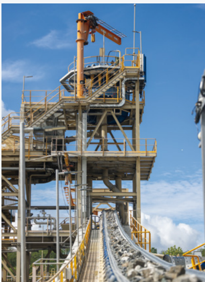
Processing Plant SAG Mill feed conveyor and Cyclone Reclassification Circuit
