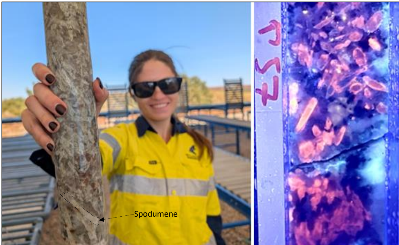
Figure 4: Diamond core from 57m in BCDD001 showing abundant elongate spodumene crystals confirmed by XRF analysis from a true width interval that returned 12.8m @ 2.0% Li 2 O from 45.3m (spodumene exhibiting bright orange fluorescence under UV light on the right hand side).
