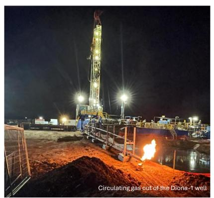
hole. Preliminary Logging While Drilling data indicates that several Permian-aged hydrocarbon bearing reservoirs are present within the Diona-1 well which warrant additional logging and testing. These preliminary observations bode well for the future potential of the well on acquisition of additional data. Drilling operations will complete followed by a wireline
