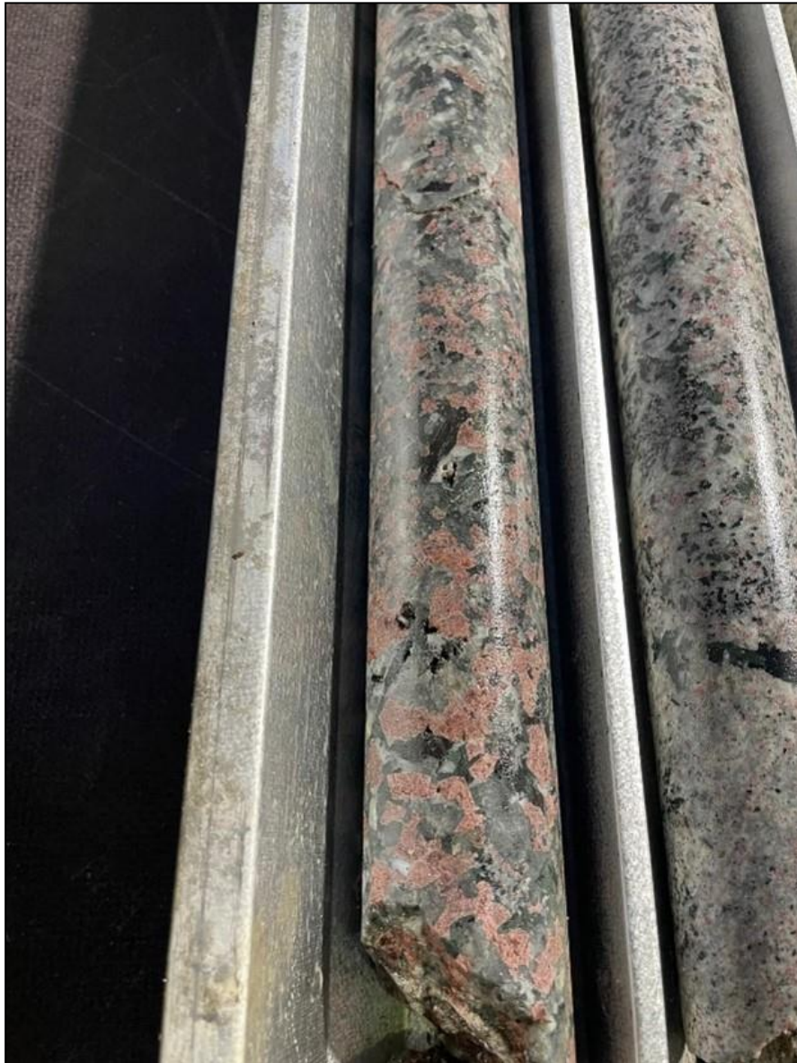
Picture 2 - Drill core with high grade eudialyte from diamond drill hole A1-24 drilled September 2024 containing 4,722.51ppm (0.47%TREO) (including 26.96% HREO" and 101.67ppm Ga2O3 "gallium oxide".
