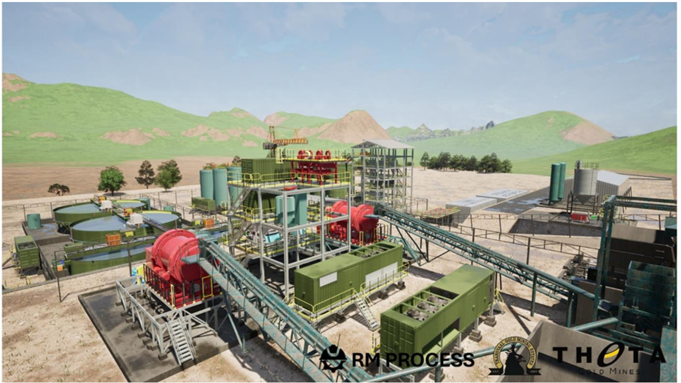
Figure 20: 3D rendering by RM Process of the Milling Circuit in Foreground
