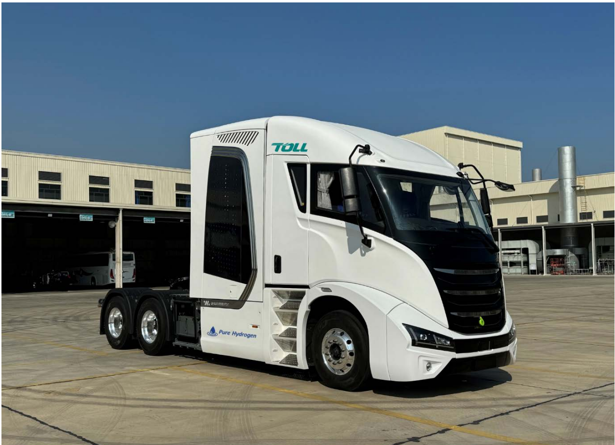
A similar version of the Taurus 70t HFC prime mover to be supplied to TOLL Transport
