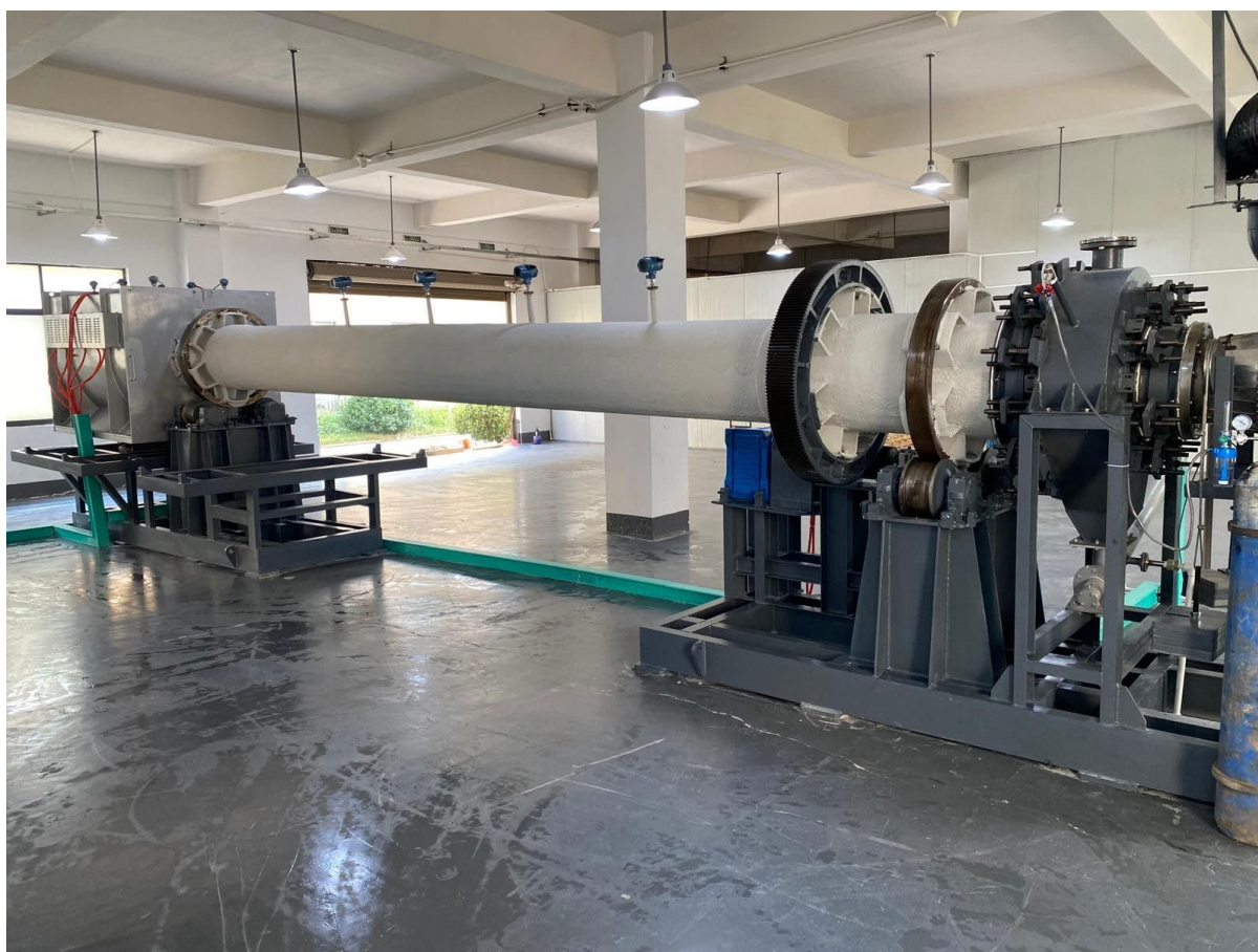
Installation of pilot scale calcining unit at Hunan Firebird Battery Technologies' Plant
