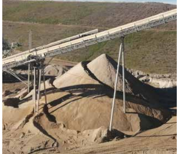
Pictured above: Stockpile showing a stockpile with multi-day feed buffer.
