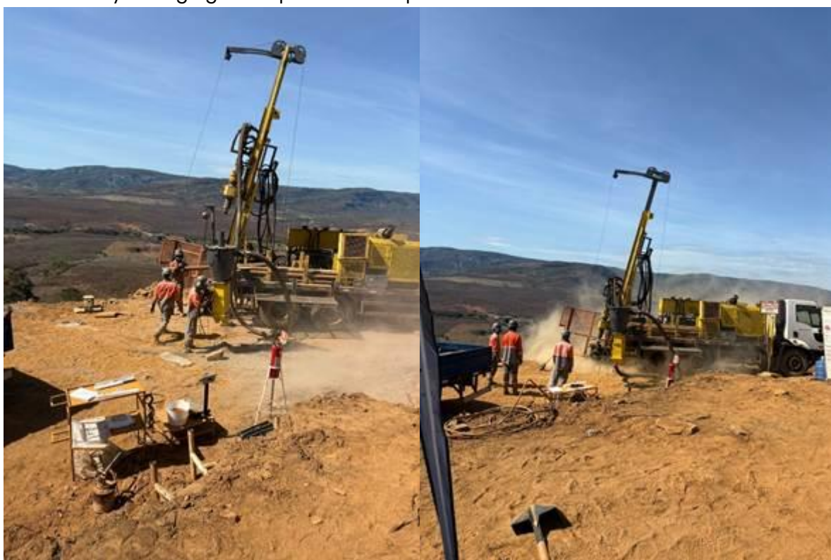
Figure 4: Image showing Reverse Circulation (RC) drilling underway at “Target 1” at the Igrejinha Lithium Project.
