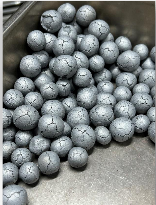
Picture 2. Pellets after Linder metallisation/reduction
