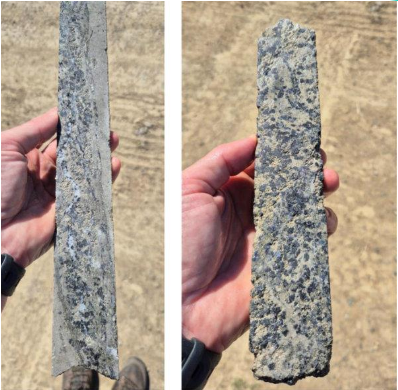
Figure 7: Photos from semi-massive sulphide zone comprising sphalerite, galena, pyrite and chalcopyrite with associated carbonate in ZRMDD064. Left – 340.55-340.98m, Right – 340.98-341.30m
