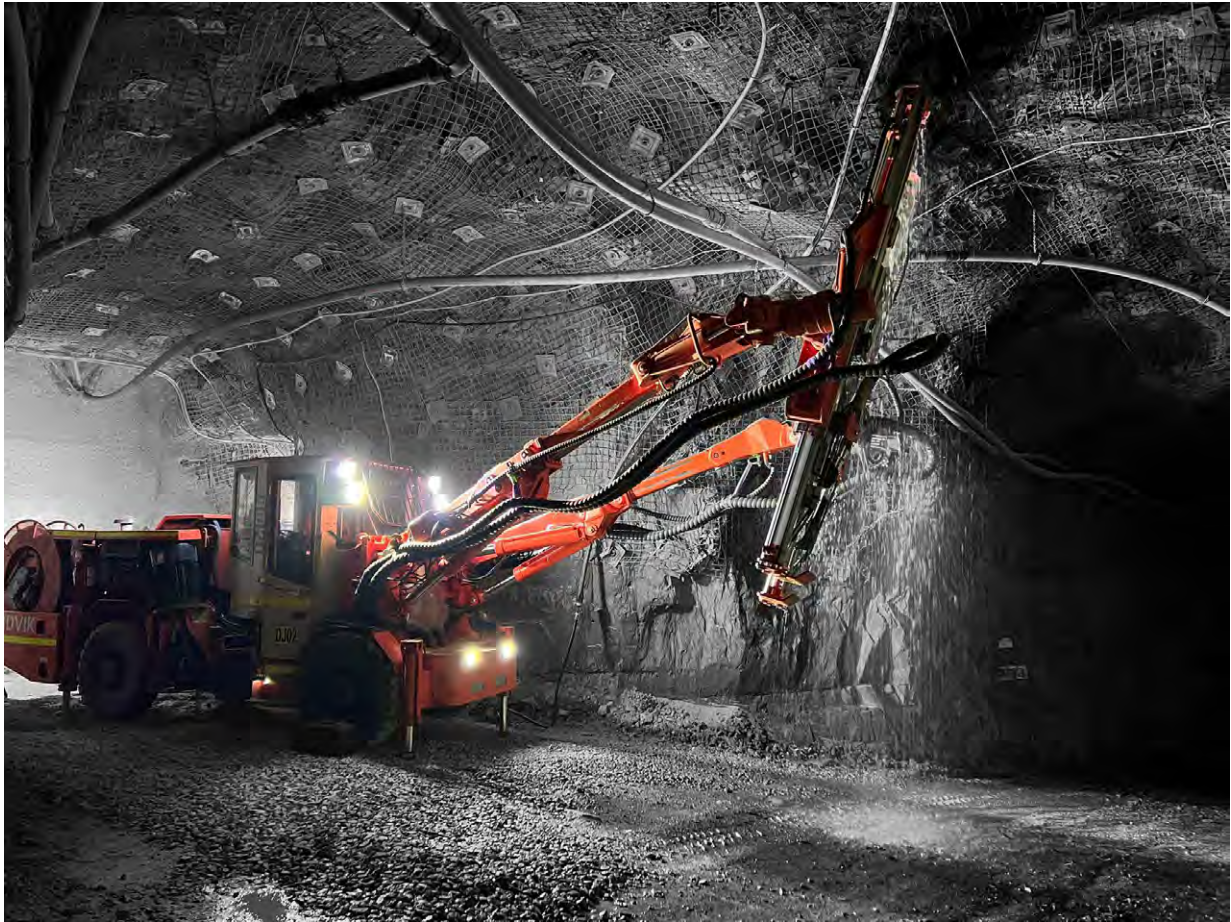
Figure 10: Meeka's first mining jumbo in operation at Andy Well.
