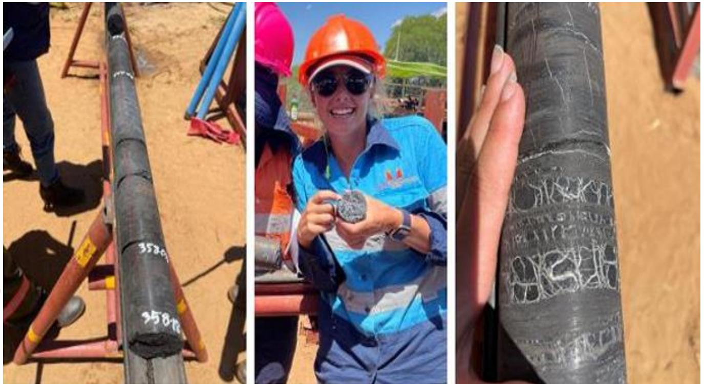
Figure 4. Serowe-3.4A Core Sampling Programme showing extensive cleats in coal
