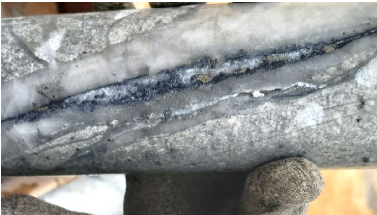
Figure 25: Photo of molybdenite + quartz + pyrite veining within quartz monzonite porphyry stock in drill hole WD22-04 (interval 640.66-642.18m downhole @ 0.22% Mo). 5
