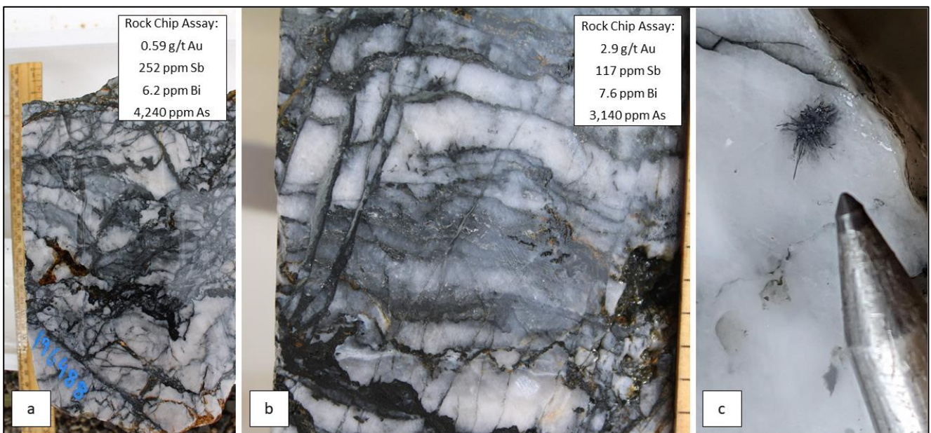
Figure 11: Rock samples collected from the Fentiman's South historic mine waste dump: (a) mineralised quartz vein with abundant stylonite and breccia textures; (b) disseminated sulphides (arsenopyrite, stibnite and pyrite) within a stylonitic and brecciated quartz vein; and (c) coarse stibnite ( \text{Sb}_2\text{S}_3 ) crystals and thin stylonites within a mineralised quartz vein 16
