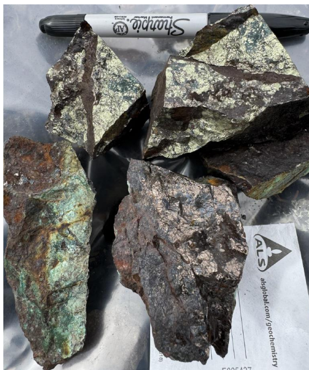
Figure 5: Photograph of sample F005437 with massive bornite-chalcopyrite which returned 42.60% Cu, 2.28g/t Au, 159g/t Ag, 0.364% Co from the Glacier IOCG trend.
