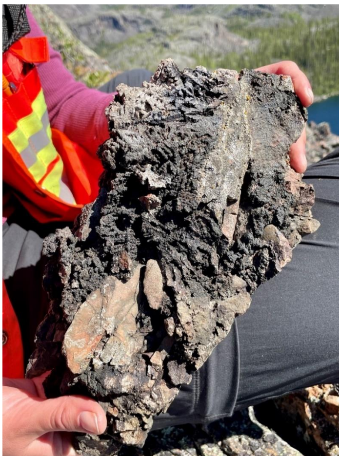
Figure 6: Photograph of sample F005909 which returned 5.35% Ag . Tarnished native silver and calcite cement can be observed between the clasts of potassic altered diorite.
