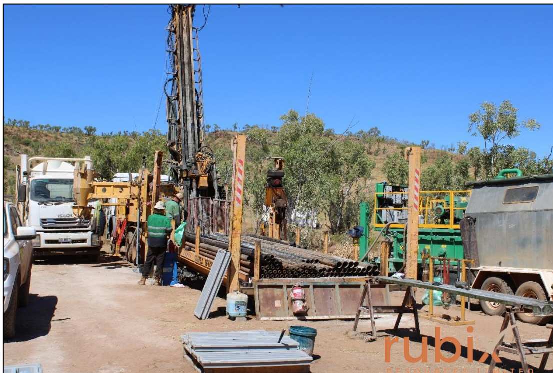
Figure 4 – Drilling at Grunter North using a multipurpose RC/DDH rig (UDR650). Green unit to the right of the rod truck is the centrifuge, which separates fines from water for recycling during drilling, significantly reducing the water requirement of drilling unless circulation is lost downhole.
