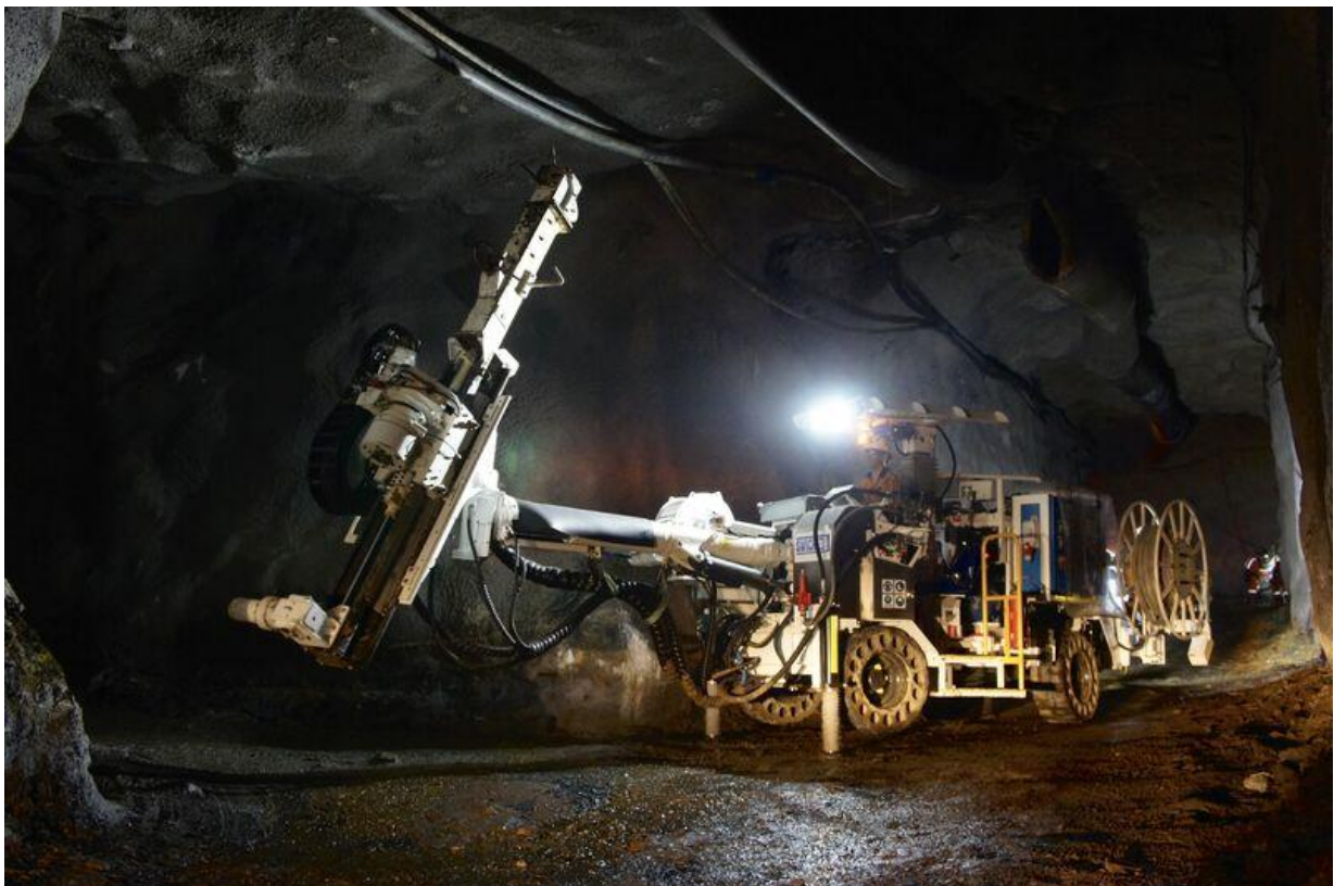
Photo 1: File photo of Swick GenII Underground Diamond Drill rig.
