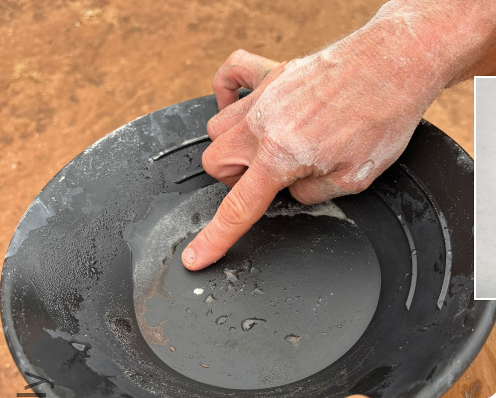
Figure 5. (Left) Panning of cassiterite grains of dark grey to black material. (Above) Collected cassiterite grains, sourced from BRC004 (108m, 7.99% Sn).
