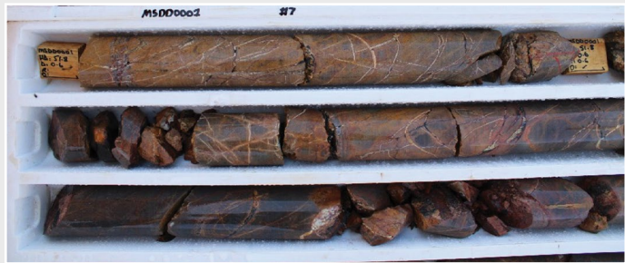
Figure 8. Hydrothermal REE mineralisation from diamond hole MSDD0001, Duchess REE Prospect, Mount Squires Project, October 2024.
