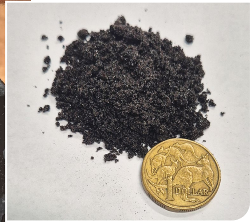
Figure 5. (Left) Panning of cassiterite grains of dark grey to black material. (Above) Collected cassiterite grains, sourced from BRC004 (108m, 7.99% Sn).
