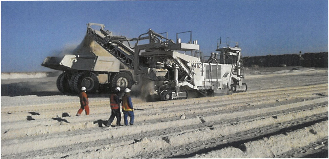
Fig 3 - Example Surface Miner – Limestone row cutting
