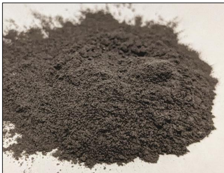
Figure 4: Antimony sulphide (37% Sb) precipitated from leach liquor 6
